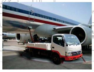
Access hatches are fitted for cleaning and maintenance of the tank unit and all work surface are covered with tread plate. Feature of the lavatory service truck includes a dual tank configuration for waste and flush water. The unit is powered by diesel engine and represent a new concept in this field with several innovative features including a driver's cabin to help position the vehicle correctly. All tanks are stainless steel and are accessible through manholes.
